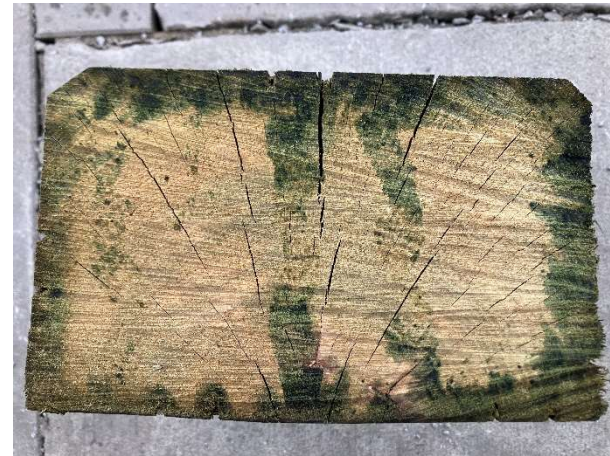
With oil based preservatives impregnated fringe area (Beech)
